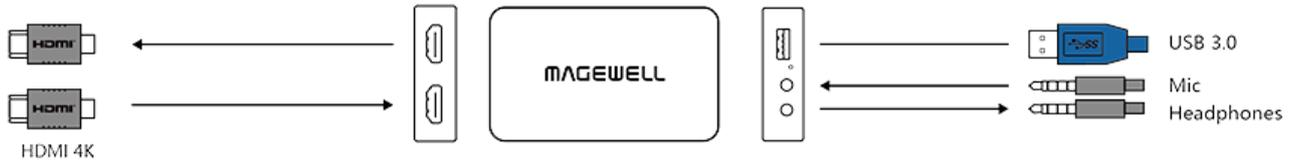
Both 4K USB Capture Plus devices support embedded audio in the SDI or HDMI input signal, as well as separate audio inputs and outputs for capture and monitoring: line-level analog input and output connections on the USB Capture SDI 4K Plus, and an analog microphone input and stereo headphone output on the HDMI model.
